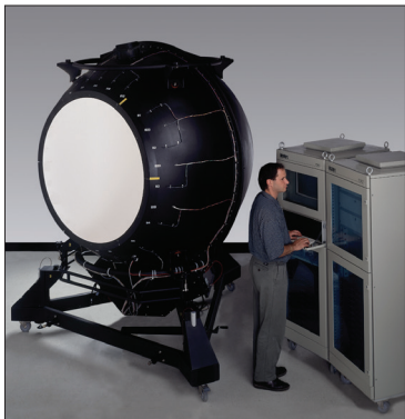
A Labsphere uniform source with a one meter aperture used for large remote sensing calibration applications.
