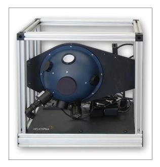
The HELIOS®Plus Sphere Assembly (HSA) is an innovative robust chassis to carry the integrating sphere and provide a home and hub for our optical and electrical components. The HSA features the Cage, a unique channeled aluminum structure designed for mounting and protection of our systems during bench top laboratory use or field use. There are (5) sphere models available to suit different sizes of apertures, spectral ranges and environmental testing needs.
