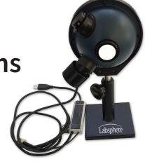
The systems provide options for laser power measurement over the 350 to 1700 nm wavelength region for optical powers ranging from nW to tens of watts. The system's calibrations are traceable to the National Institute of Standards and Technology (NIST).
